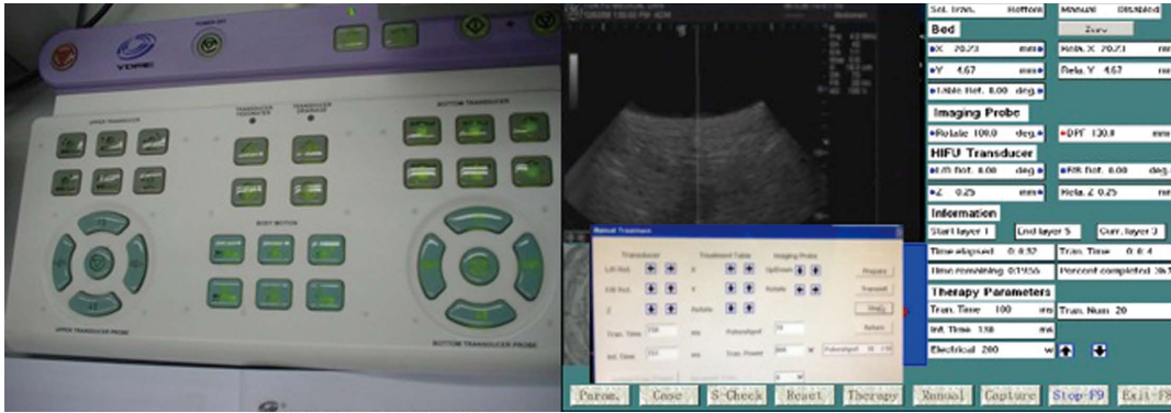
Figure 5 Monitoring system and treatment table. The B-mode ultrasound was used to define the target area, therapeutic range, therapeutic layers, and power. The whole procedure of the treatment and the shift of focus were automatically controlled by computer.
